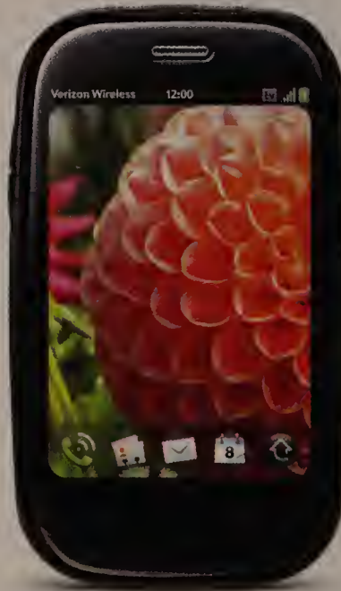
THE PRE PLUS has a touch area instead of a hardware button.
